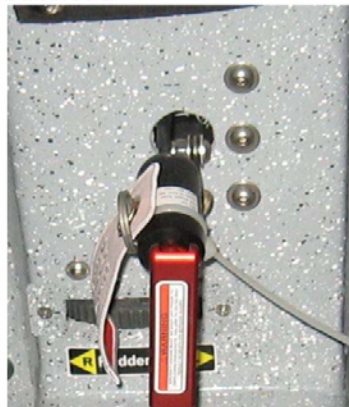
Fig. 2: New BRS rescue system handle installation which is not affected by this TA
