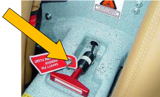
Fig. 1 – Sample view of BRS activation handle in a CTLS with locking pin inserted – other systems and aircraft models comparable.
