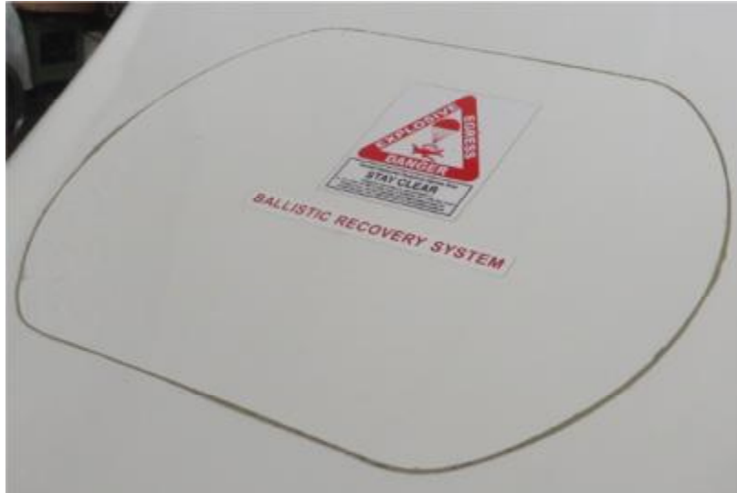
Fig. 5 – Sample view correct application of warning label provided by BRS
