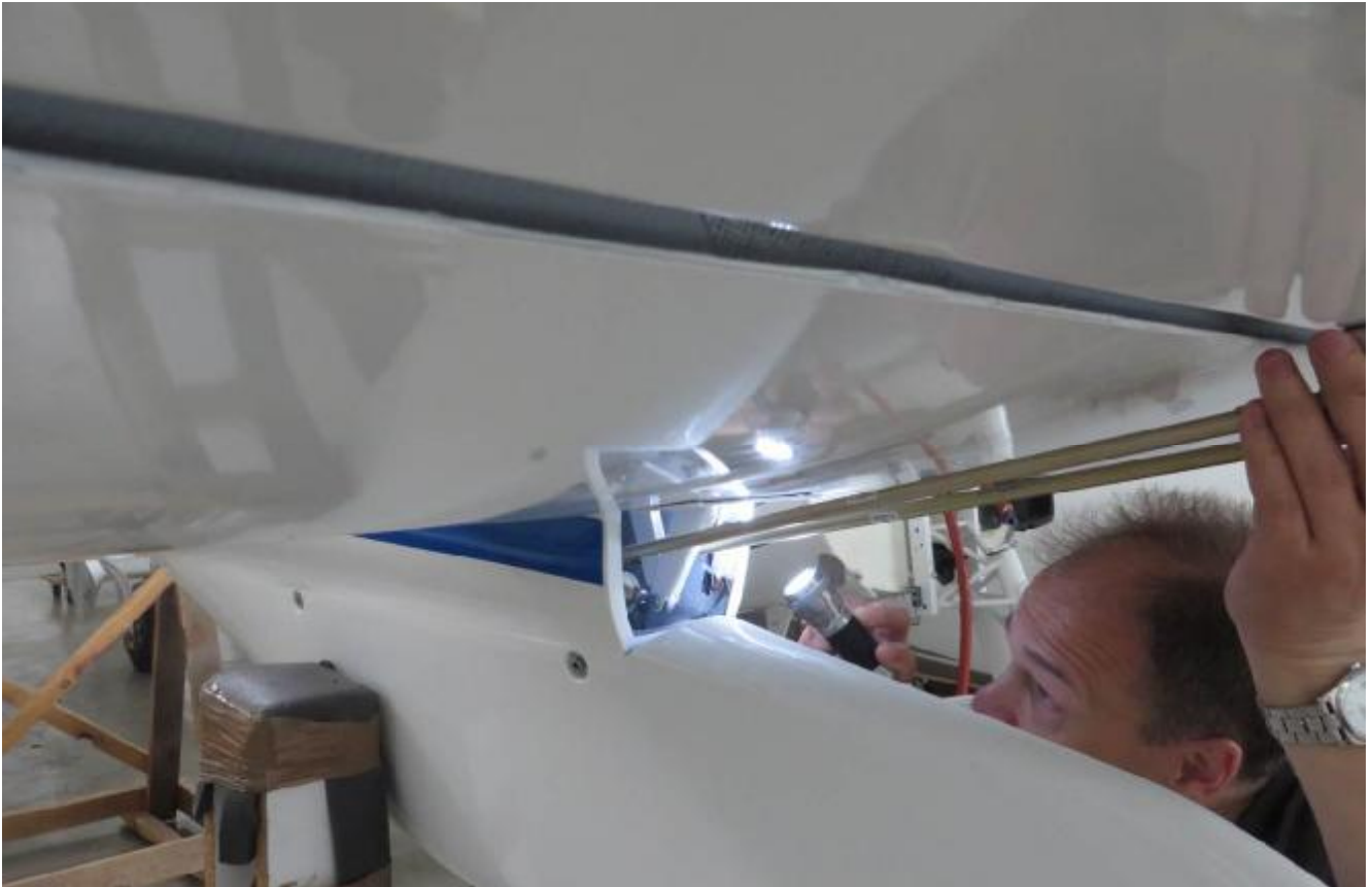
Fig. 4 – Inspection of stabilator mounting pivot.
